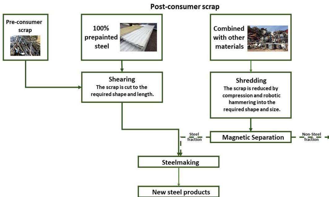
Figure 2. Recycling routes for pre-painted steel
