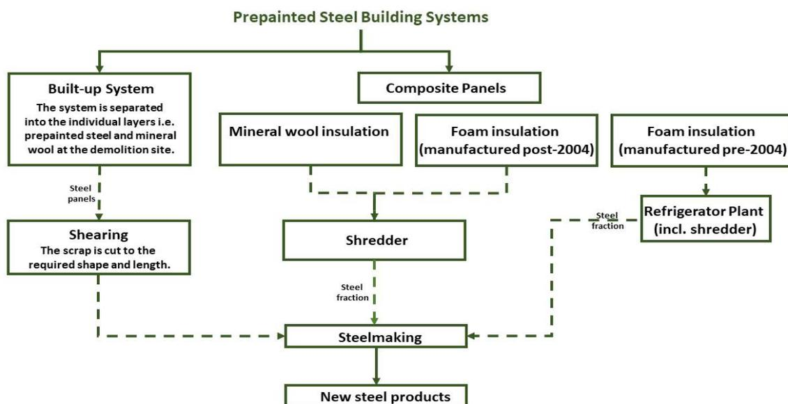
Figure 3. Recycling routes for prepainted steel building panels
