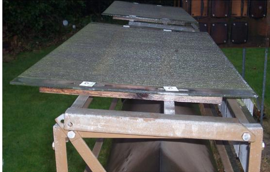
The T29 test can be undertaken using modified ECCA exposure racks as shown in **Fig. 1**. The area normally used to expose panels at the 5°S orientation has a grooved collector plate installed which collects dirt and rainwater and directs it onto test samples installed on the upper row of the 90°N exposure aspect.
