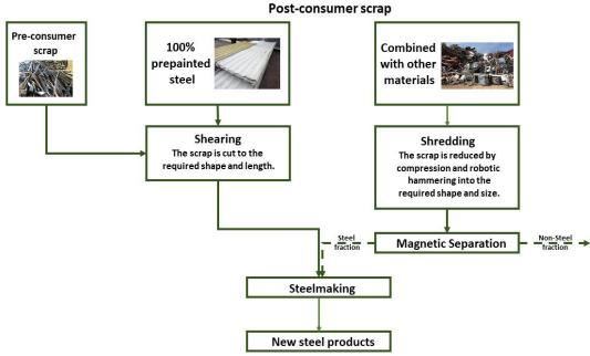
Figure 2. Recycling routes for prepainted steel
